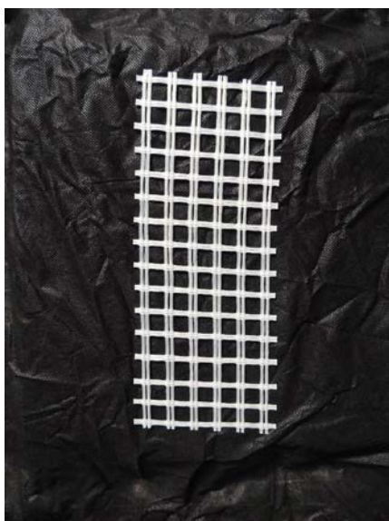
Fig. 3: AR glass reinforcement
