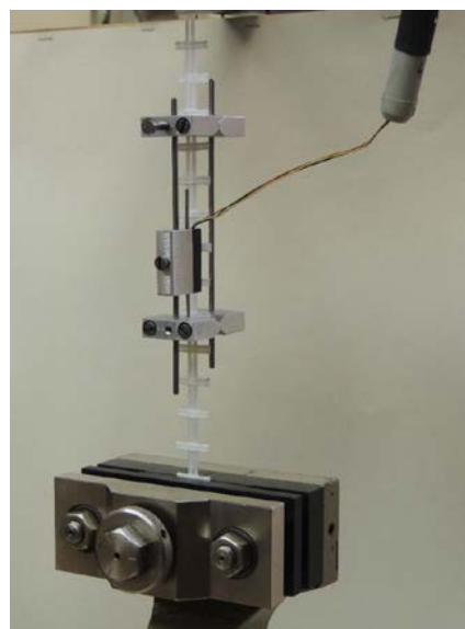
Fig. 4: Testing of AR glass reinforcement
