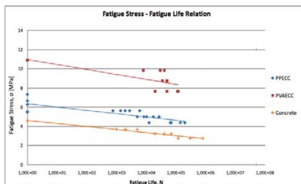
Fig. 4: Flexural stress – fatigue life relation for PVAECC, PPECC and conventional concrete
