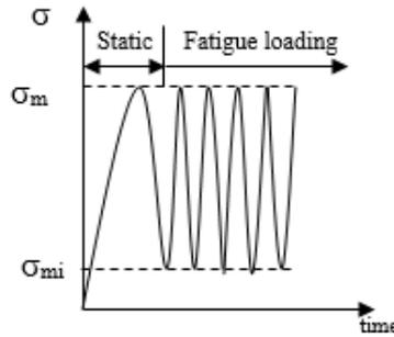
Fig.1: Loading pattern for fatigue test
