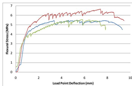
Fig. 2: Flexural behavior of PPECC
