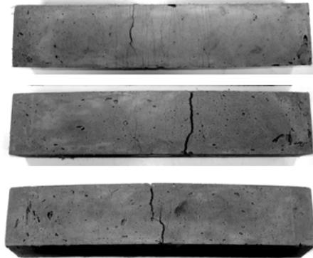
Fig. 5: Crack pattern for PPECC specimens under monotonic and fatigue loading at  $0,8\sigma_{ult}$  e  $0,7\sigma_{ult}$ , respectively
