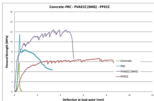
Fig. 3: Comparison of concrete, PPECC, PVAECC and FRC typical flexural behavior
