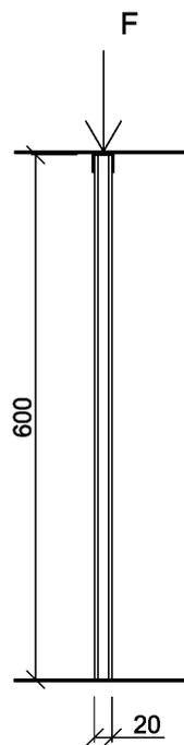
Figure 6: A compression buckling test.
