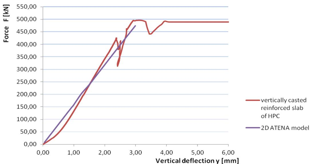
Figure 11: The comparison of the test results and model in ATENA program.
