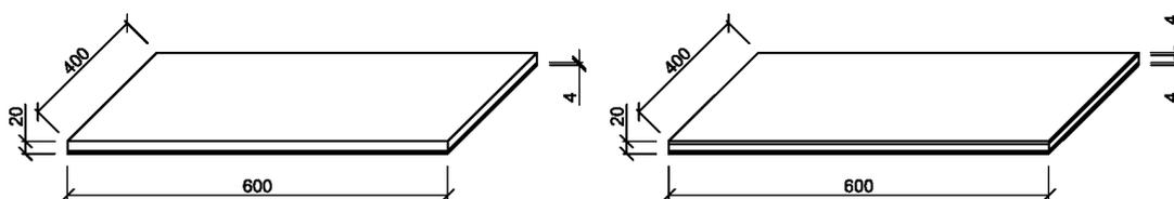
Figure 1: Position of fabric in specimens.
