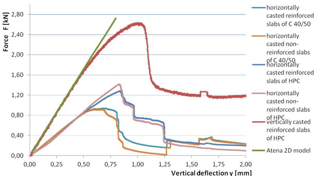
Figure 8: The comparison of average test results and model in ATENA 2D program.
