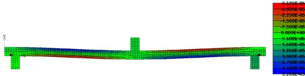
Figure 9: A displacement of the bending test model in ATENA program.
