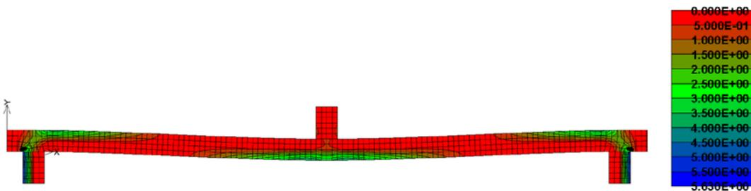
Figure 10: A principal stress of the bending test model in ATENA program.
