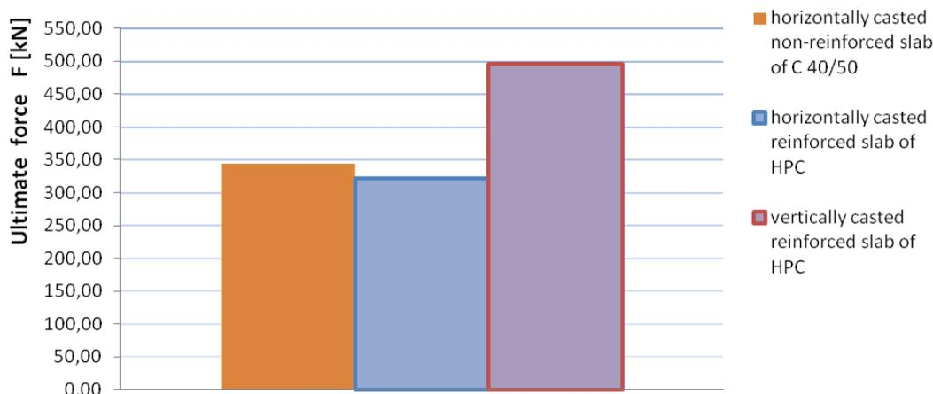
Figure 7: The comparison of the average results in the compression buckling test.
