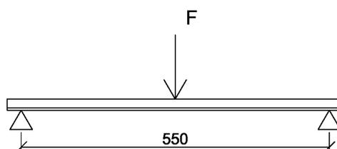
Figure 4: A three-point bending test.
