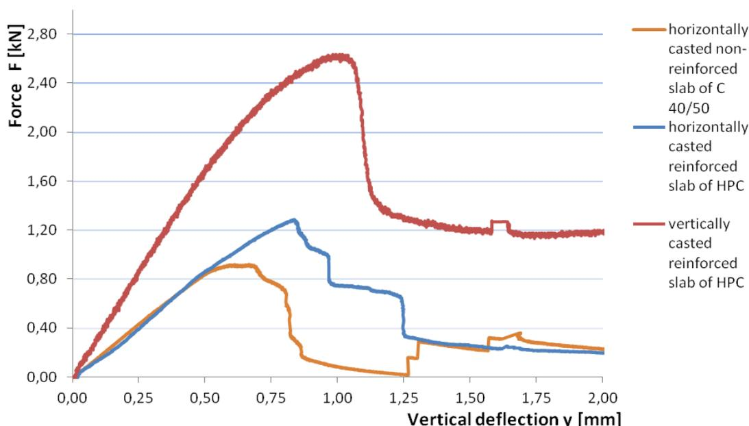
Figure 5: The comparison of the average results in the three-point bending test.
