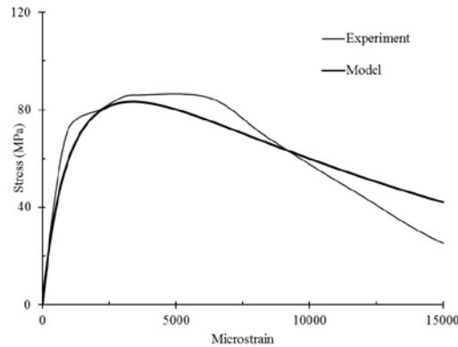
Fig. 3: Comparison of experimental and predicted stress-strain relationship for plain concrete mix at strain rate of  $78 \text{ s}^{-1}$ .
