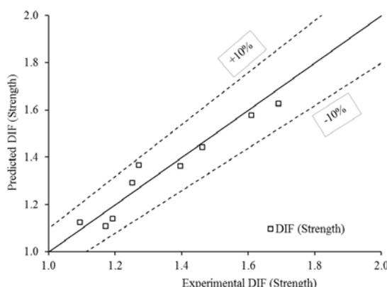
Fig. 2: Scatter in the prediction of DIF (strength) using Eq. (17).
