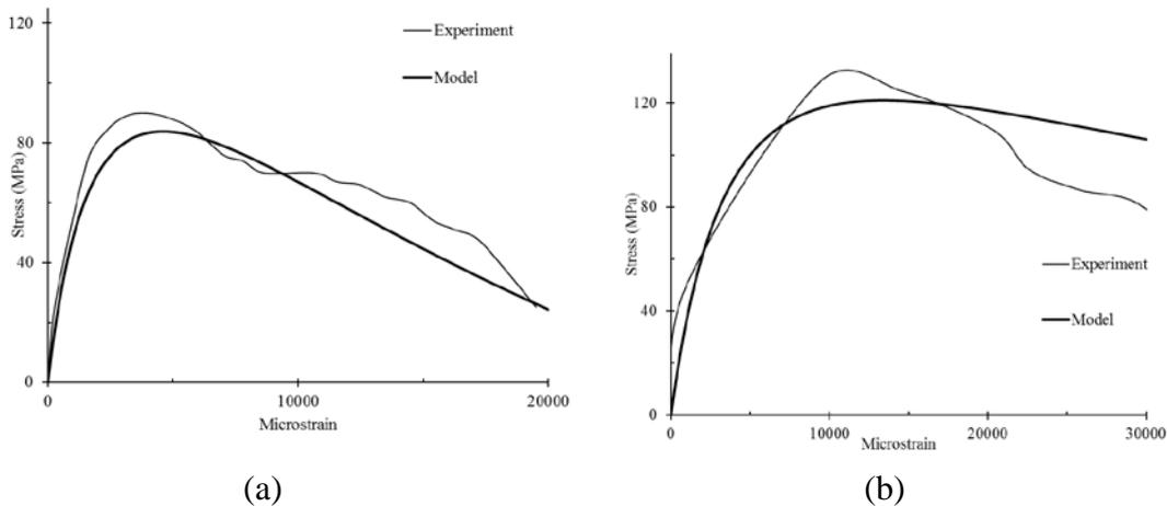
Fig. 4: Comparison of experimental and predicted stress-strain relationship for fibre reinforced concrete: (a) Mix M1 at strain rate of  $32 \text{ s}^{-1}$ ; (b) Mix M2 at strain rate of  $112 \text{ s}^{-1}$ .
