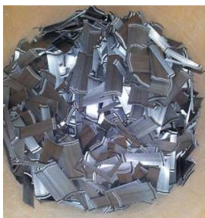
Fig.2: Hooked-steel fibres used in the study.
