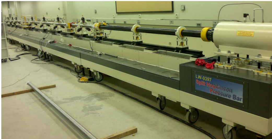
Fig.1: Schematic (a) as well as the experimental setup (b) of SHPB.
