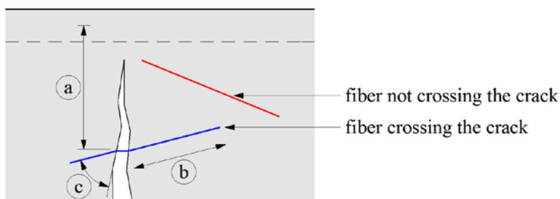
Fig. 1: Parameters of a discrete fibre
