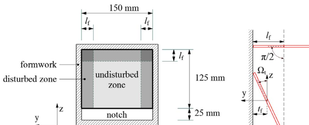
Fig. 4: Wall-effect of the formwork
