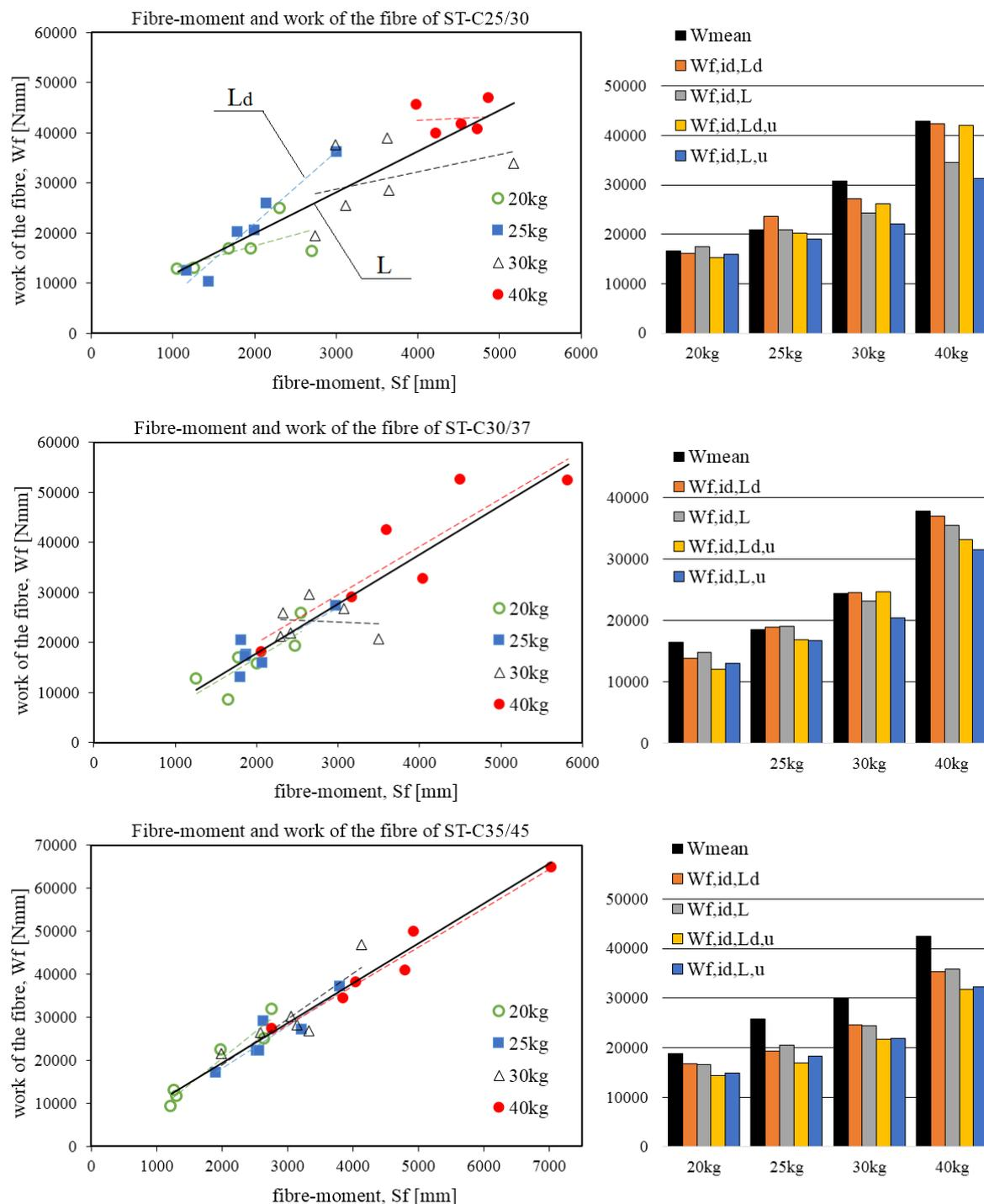
Fig. 7: Fibre-work and work of the fibre relationships with the evaluations
