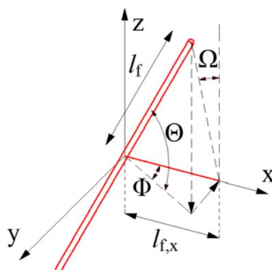
Fig. 3: Length of the fibre in the direction x
