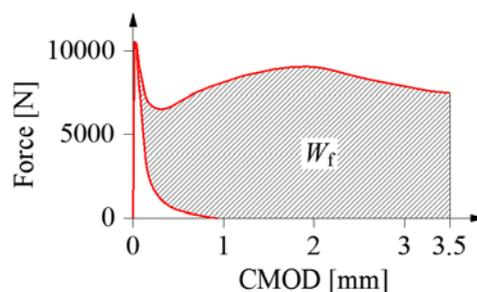
Fig. 6: Fibre-work
