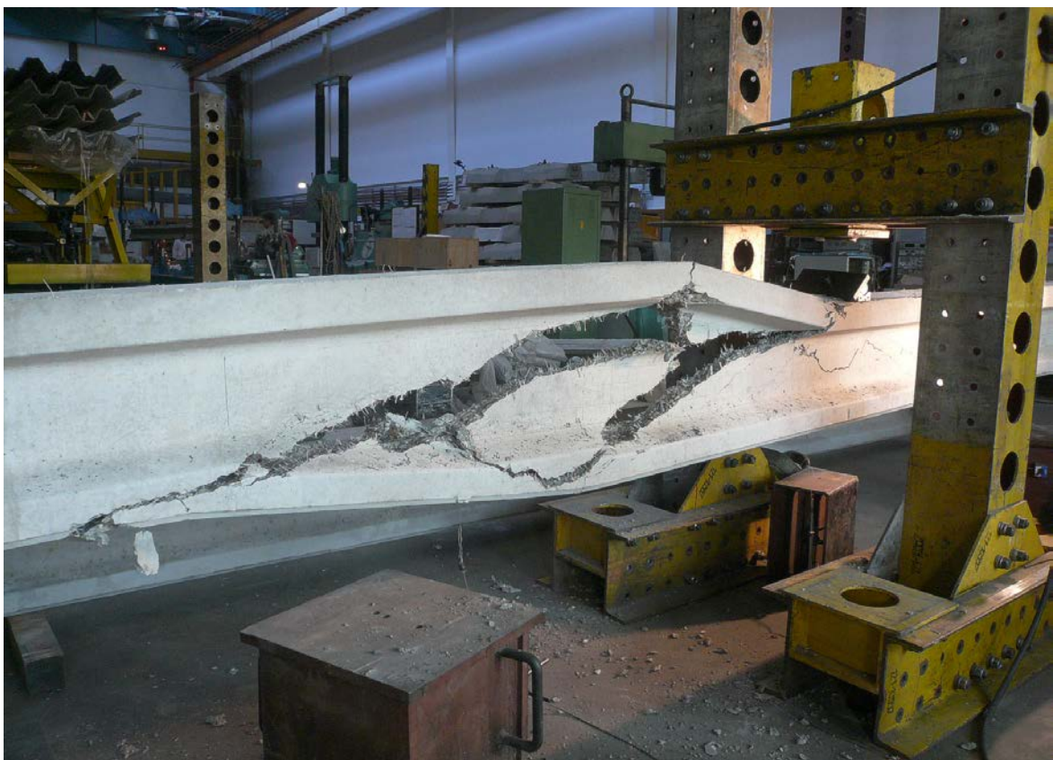
Fig. 3: Shear failure of the 8000/1 beam specimen
