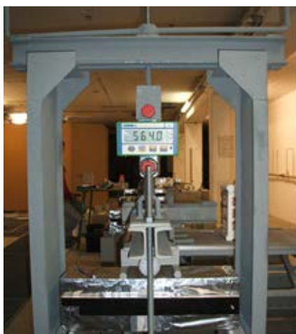
Fig. 4: Applying the exact creep load. (Note: supporting rollers in this equipment, not sufficient moveable, instead lubricants are used)
