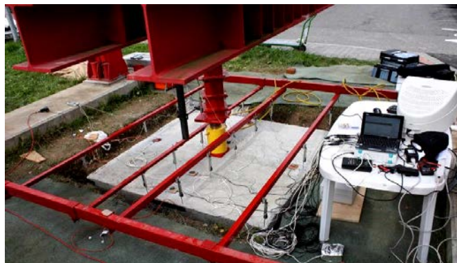
Fig. 2: Load test of the fibre concrete slab
