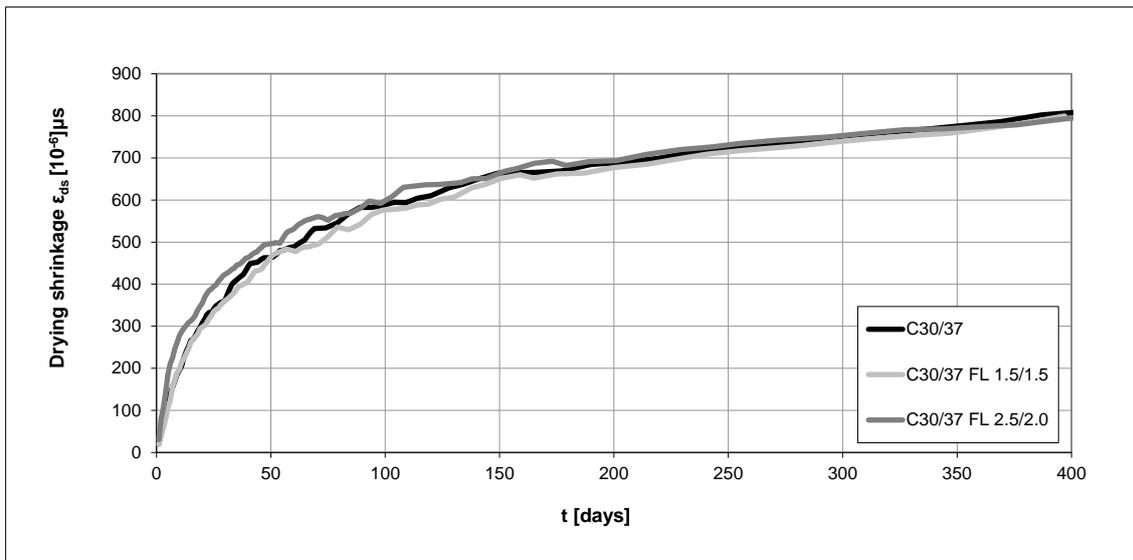
Fig. 5: Drying shrinkage strain for the three concrete types
