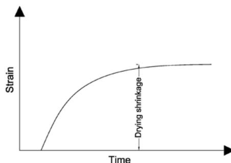
Fig. 1: Drying shrinkage
