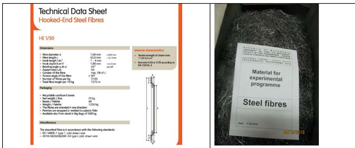
Fig. 2: Technical data sheet of the used fibres
