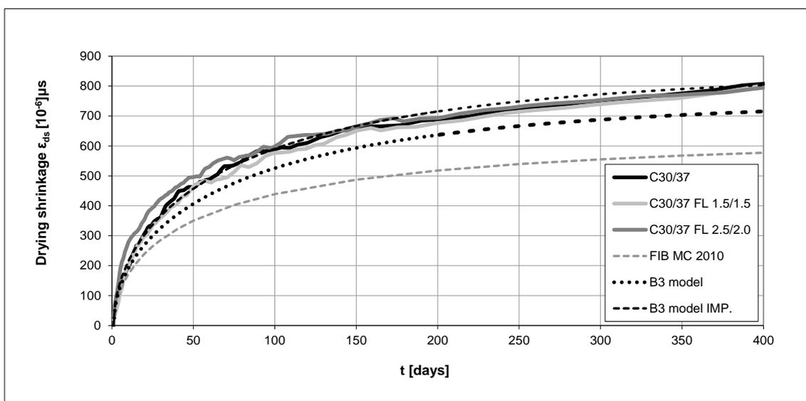
Fig. 6: Experimental and analytical results for drying shrinkage up to age of 400 days
