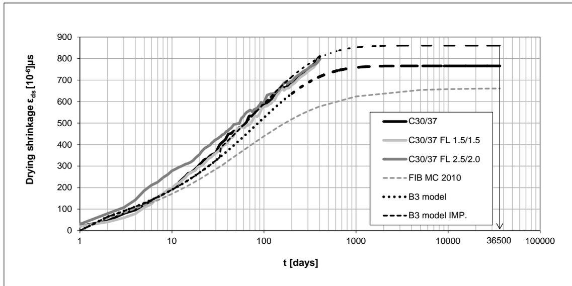
Fig. 7: Experimental and analytical results for drying shrinkage up to age of 100 years in logarithmic scale
