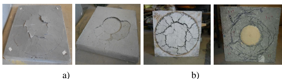
Figure 8. View of the bottom (L) and top (R) of specimens of a) DHCC and b) HPFRC
