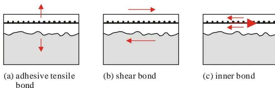
Fig. 1: Bond failure modes of a TRC strengthening applied to a RC surface
