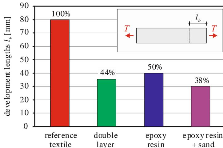
Fig. 6: Comparison of the development lengths
