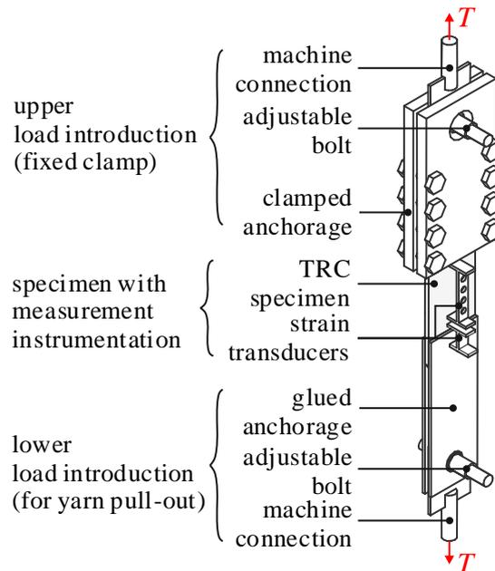
Fig. 2: Test setup for the development length of the textile (textile pull-out test)
