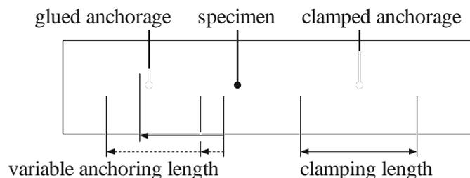
Fig. 3: Specimen for adaptive testing of textile's development length
