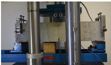
Equipment to Residual Tensile Strength by Bending in Concrete Beams Reinforced with Steel Fiber and Sketch picture of three-point bending beam specimen, measures in mm FIC-UANL-MEX.
