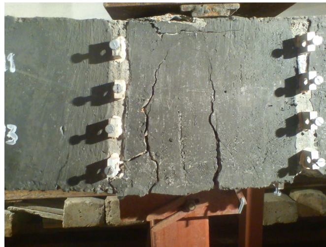
Fig. 7 The fracture of the girder
