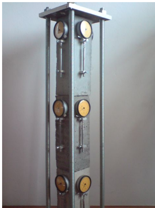
Fig. 3 The prisms with the deformeters
