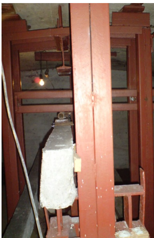
Fig.1 The device for the measuring of the load on the girders
