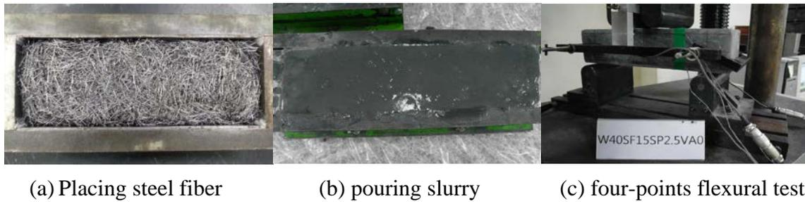
Fig. 3: Specimen fabrication procedure and four-points flexural test
