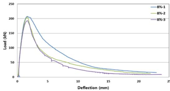
Fig. 6: Load-deflection curve with 8.0% steel fiber volume fraction
