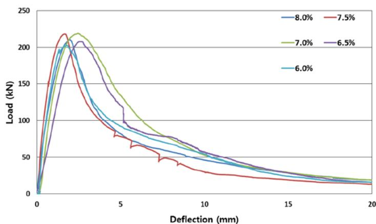
Fig. 5: Load-mid span deflection curve with respect to steel fiber volume fraction
