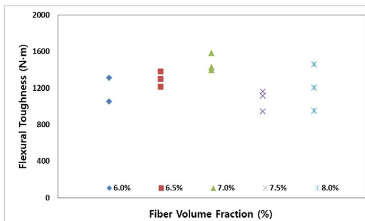
Fig. 13: Test results of flexural toughness according to the steel fiber volume fraction
