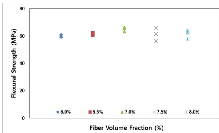
Fig. 12: Test results of flexural strength according to the steel fiber volume fraction
