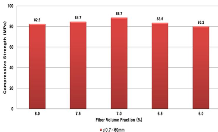
Fig. 14: Test results of compressive strength according to the steel fiber volume fraction
