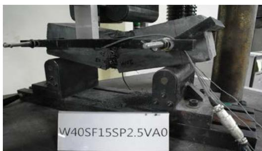
Fig. 11: High ductile behaviour in flexural test
