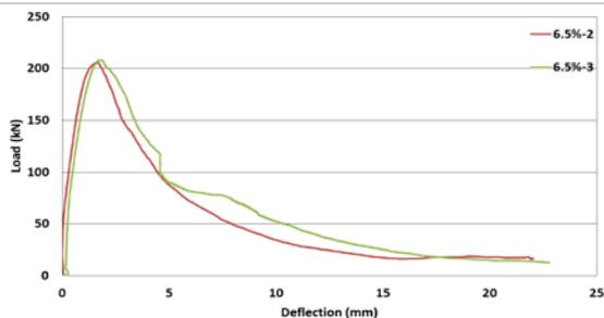
Fig. 9: Load-deflection curve with 6.5% steel fiber volume fraction
