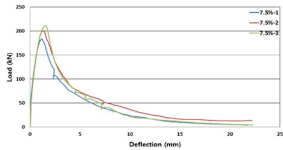
Fig. 7: Load-deflection curve with 7.5% steel fiber volume fraction
