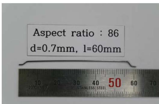
Fig. 2: Type of steel fiber (aspect ratio 86)
