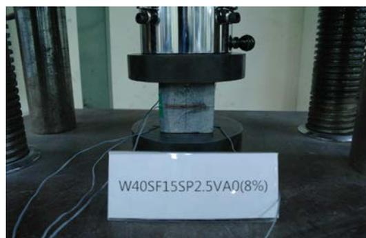
Fig. 4: Set-up of the experiment on compressive strength
