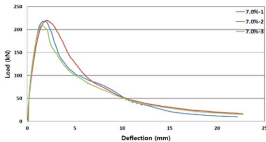
Fig. 8: Load-deflection curve with 7.0% steel fiber volume fraction
