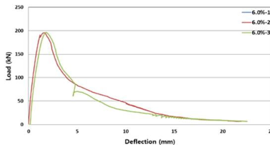
Fig. 10: Load-deflection curve with 6.5% steel fiber volume fraction
