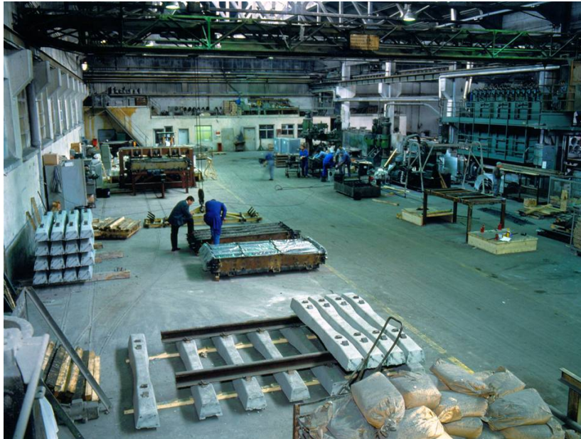
Fig. 2: Pilot production of PCS-SFRC.
