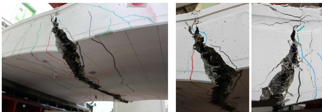
Fig. 7: Crack openings at the end of the bending test
