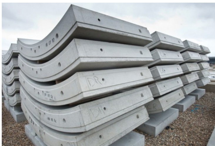
Fig. 2: Tunnel lining segments reinforced by ArcelorMittal steel fibres HE ++90/60 – Crossrail London
