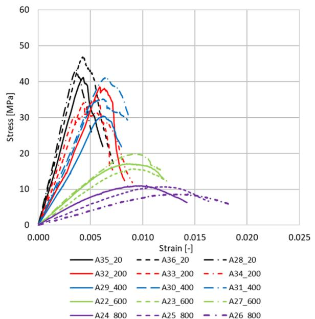
Figure 3 – Stress-strain diagrams of air-entrained concrete
