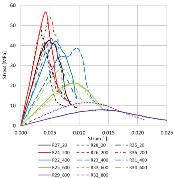
Figure 2 – Stress-strain diagrams of reference concrete
