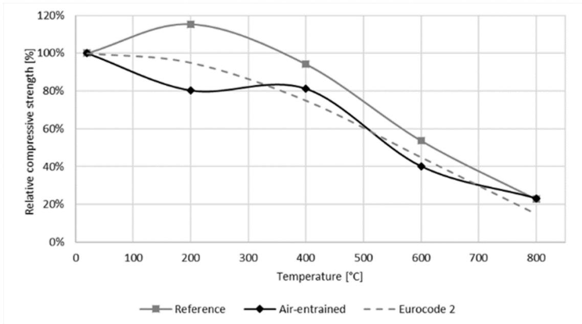
Figure 4 – Relative mean strength of reference concrete and air-entrained concrete at various temperatures compared to Eurocode 2 recommended values
