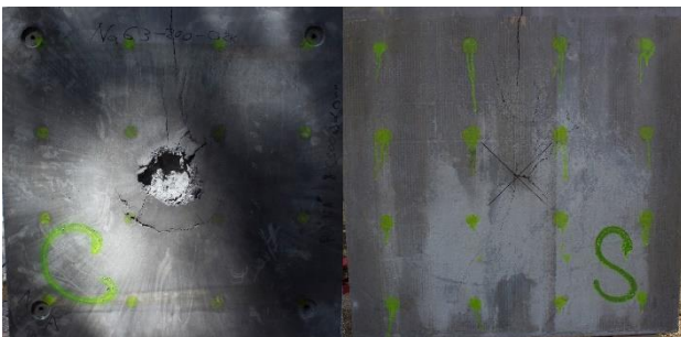
Fig. 5: Specimen Nr. 28 contact side (left) and soffit (right).
