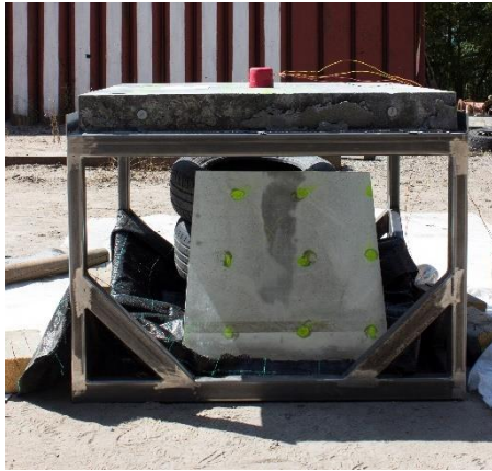
Fig. 2: Specimen with the explosive charge and mirror under specimen.
