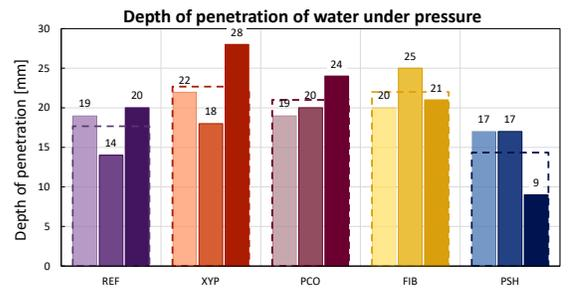
Figure 6: Depth of penetration of water under pressure for different concrete mixes.
