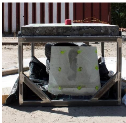
Fig. 1: Specimen with the explosive charge and mirror under specimen.
