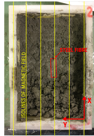
Figure 9: Steel fibre after alignment, revealed.
