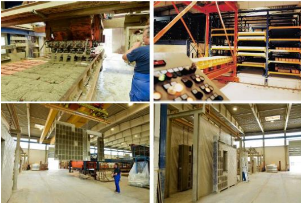
Figure 9: The production of precast wall panel RZEH® (Rötzer® Ziegel Element Haus/Das Werk/Fertigung ©n.d.)
