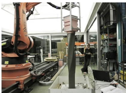
Obr. 7: Metoda Smart Dynamic Casting
