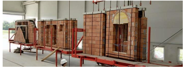
Figure 8: The made Rimatem® panels with Vario-traverse on the transport container (Rimatem®/sakha-prom ©n.d.)
