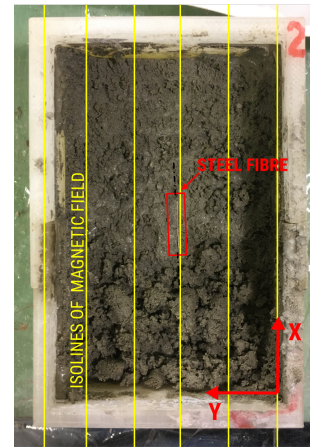
Figure 9: Steel fibre after alignment, revealed.
