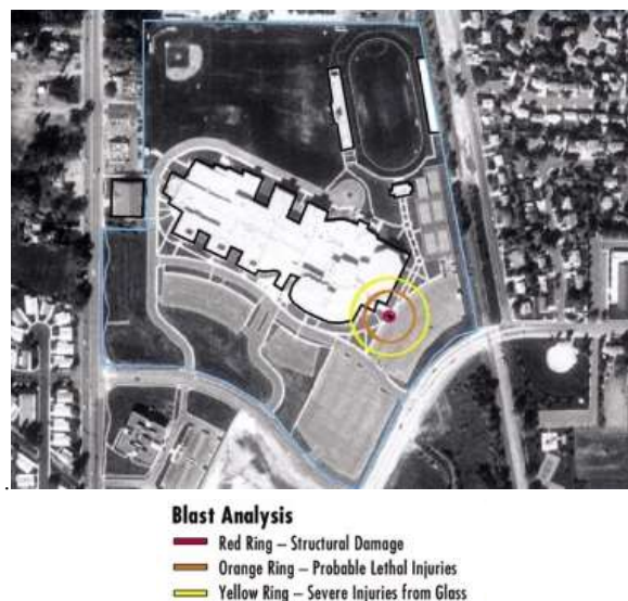
Figure 1: Blast analysis of a building for a typical car bomb detonated in the building's parking lot. Red radius = 4.5 m, orange radius = 22.5 m and yellow radius = 30 m (FEMA-426/BIPS-06 2011).
