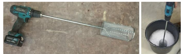
Figure 1: Foam preparation setup.
