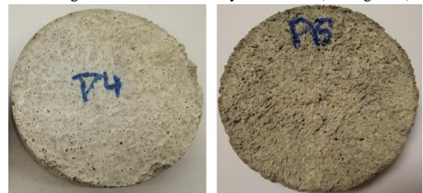
Figure 4: Visual difference between the reference sample (PR = P4) and sample P6.
