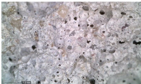
Figure 5: Microscope image of sample P8, magnification 50 \times .
