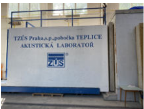
(e) Wall specimens placed between the testing rooms.
