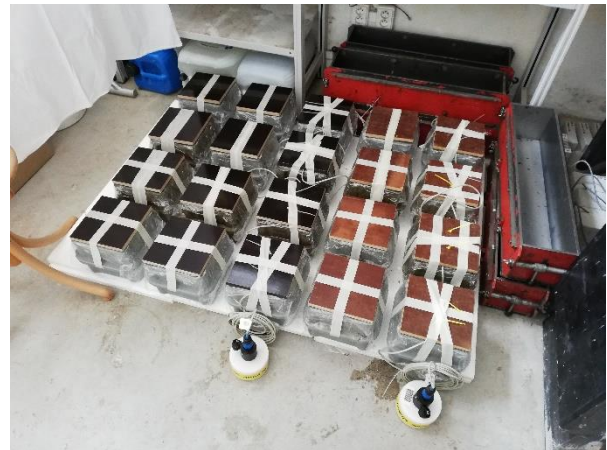
Figure 5 - Early-age compressive strength samples [photo: author]
