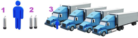
Figure 1: Visualisation of 3 compression use cases with a same amount of hydrogen – 5 kg. From the left – 700 bar, 350 bar and 1 bar. Visualized by the author.
