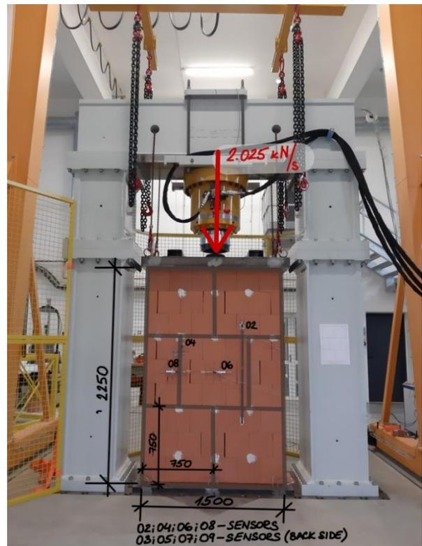
Figure 7: Test scheme for determining the compressive strength of masonry
