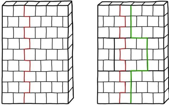
Figure 6: Bond(s) of masonry in traditional masonry wall and in wall of small-format precast units
