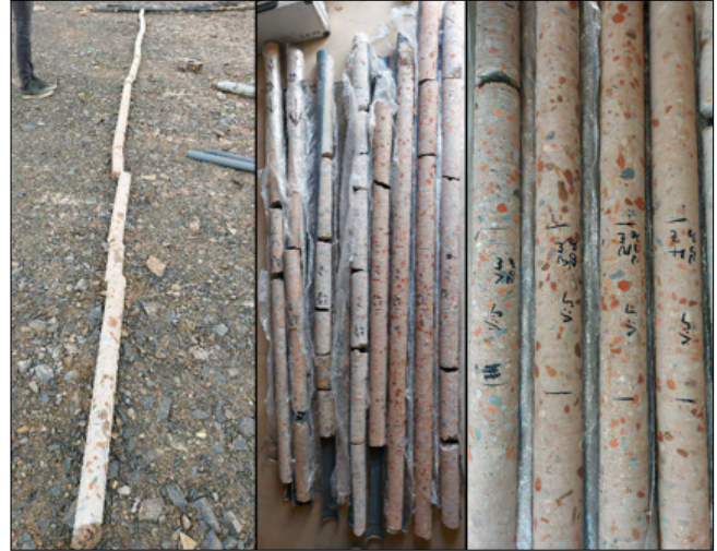
Figure 5: Test boreholes from bored piles made of recycled aggregate concrete containing 50% recycled aggregate.
