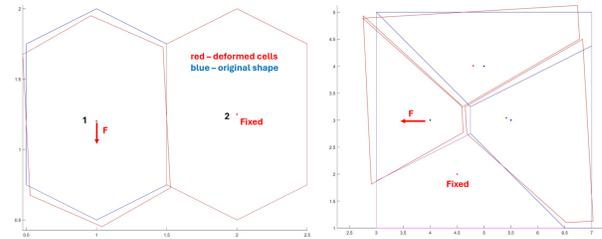
Figure 9: Simple configuration of Voronoi cells to test the calculation
