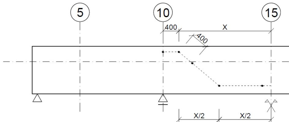
Parabolic shape of tendon is approximated using circular arcs and straight lines. The lines drawn in the previous step are tangent to circular arcs of the tendon.
