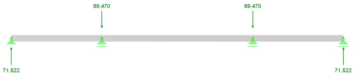
The vertical reactions should be balanced which means they should be of the same value. The inaccuracies in this case are caused by rounding of the subresults during the calculation. For further use, the average value of reactions will be used:
