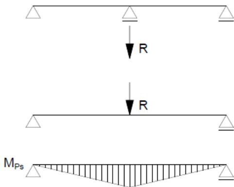
The design of the prestress must consider both moment from external loading and secondary moment from prestressing  $M_f + M_{ps}$ :
