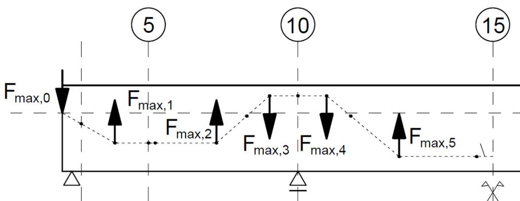
The vertical forces caused by prestressing at the points of tangent intersection and corresponding equivalent loading will be determined for the state without losses of prestress (input state, where the forces and stresses are at their maximum). That means the prestressing force in the tendon is:
