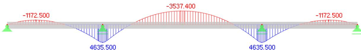
(Notice: The bending moment  $M_p$  includes both primary bending moment  $M_{pp}$  and secondary bending moment  $M_{ps}$ .)
