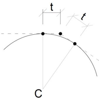
Then, the centre of the circle can be found as an intersection of two lines that are perpendicular to the tangents at the contact points.
