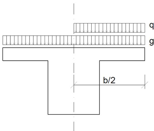
The dead load is symmetrical, which means its effect on the torsion is zero.
