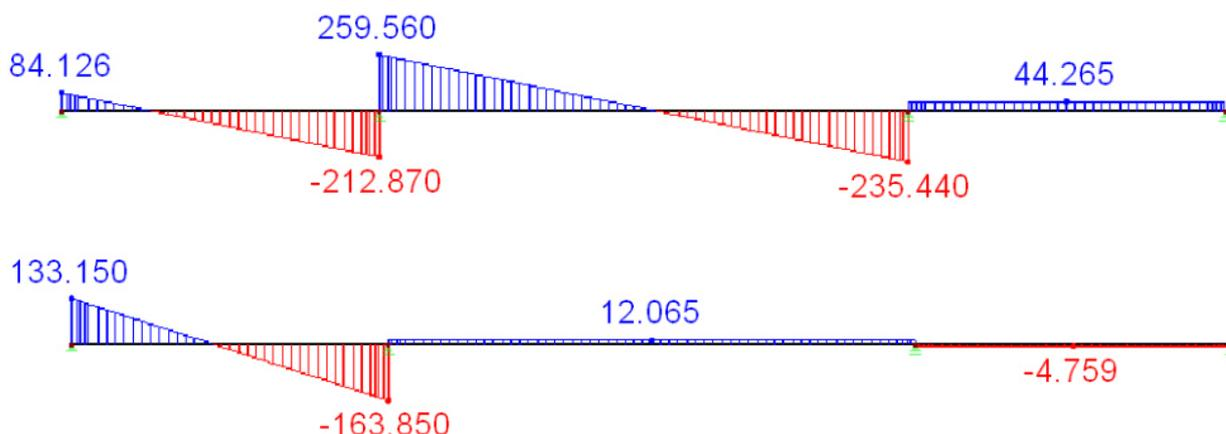
The maximal characteristic values of shear force of LC3 – LC6:
