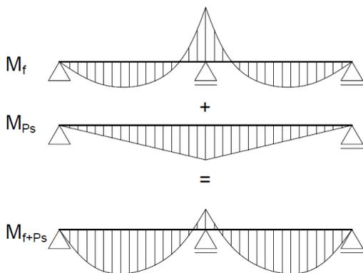
As the structure is statically indefinite, secondary prestressing moments are created (moment diagram in the picture below). Firstly, its maximal value is estimated.
