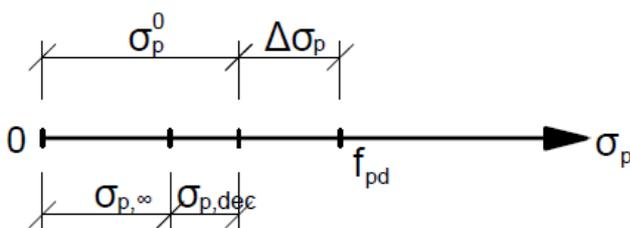
The reserve stress  $\Delta\sigma_p$  is variable – when it is zero, the total stress is equal to  $\sigma_p^0$ ; when it is at its maximum, total stress is equal to  $f_{pd}$ .
