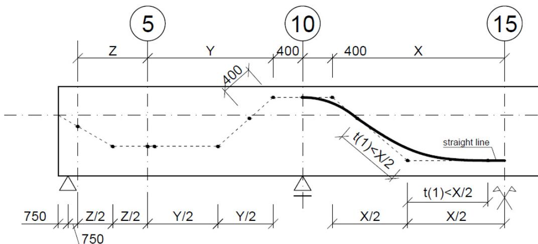
To draw the tendon shape to the left from the cross-section 10, use analogical procedure as in previous steps. The lowest point of the lower arch must be placed in the position of maximal bending moment  $M_5$ . Notice that the first 1500 mm of the tendon must be straight. Due to the geometry of the beam, there is a straight part of the tendon before the concave arc.
