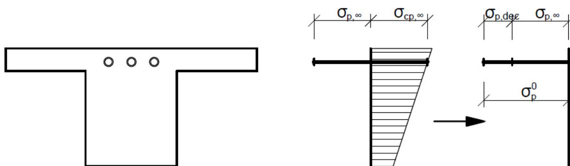
If the compression in concrete should be eliminated from to zero, the tension in the reinforcement must be proportionally increased from  $\sigma_{p,\infty}$  to  $\sigma_p^0$  by  $\sigma_{p,dec}$ .
