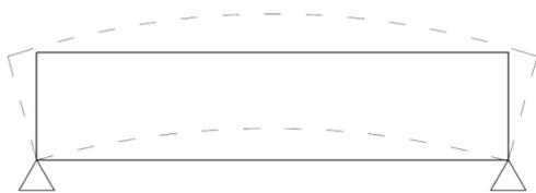
However, the middle support is present and fixes the beam in its original position. This fixation causes a reaction  $R$  in the support. This reaction applied as a loading force to the beam creates the secondary prestressing moment  $M_{ps}$ :
