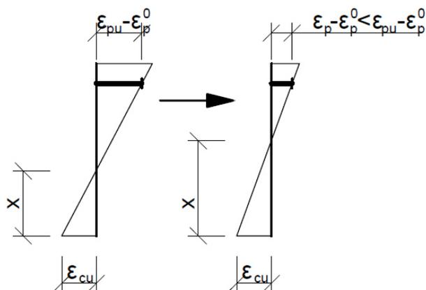
If the force  $F_c$  would have exceeded the sum of  $\Delta F_p$  and  $N_p^0$ , it would have been necessary to lower it and, therefore, lower the  $x$ . In that case, the strain of the reinforcement would have remained fixed on its limit value  $\varepsilon_{pu}$  and the strain of concrete would have been lowered.
