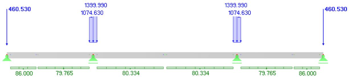
The bending moment caused by the equivalent load is the bending moment of prestressing  $M_{p,max}$  (before losses of prestress):
